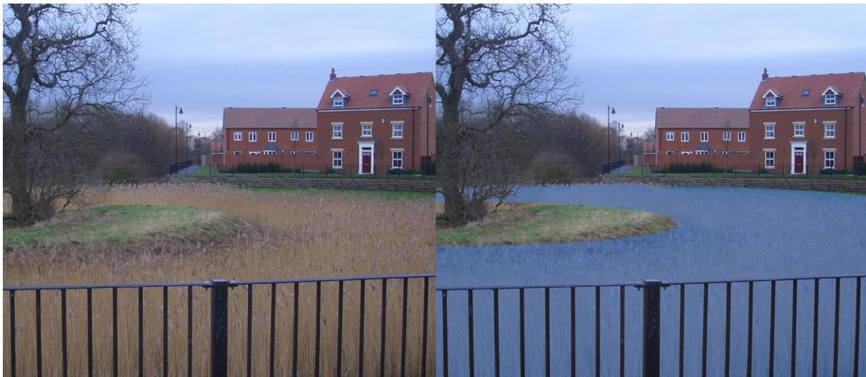
**Figure 10:** The Great Park Development, UK has green natural spaces that are designed flood with excessive storm water.
