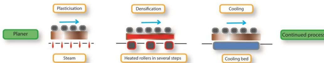
Figure 5. Schematic illustration of a continuous surface densification process (from Sandberg et al. 2017)
