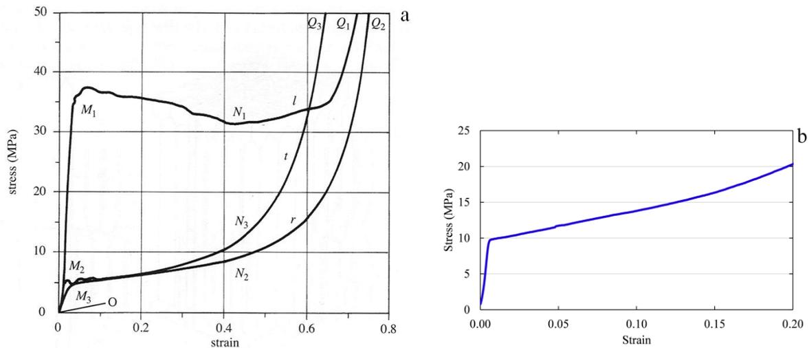
**Figure 2.** Stress-strain curves of samples of poplar (a) of dimensions 25x25x5 mm<sup>3</sup> subjected to compression in the l, r, t directions under controlled displacement at a rate of 1 mm/min (Navi and Sandberg 2012), and oak (b) subjected to controlled compression in the longitudinal direction (based on Báder and Németh 2018)
