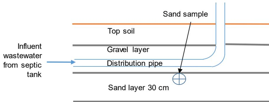
**Figure 1** Typical design of a drain field and location where sand was sampled
