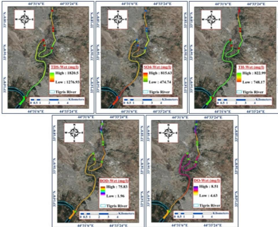
**Figure 4** Maps of the spatial distribution of concentrations for wet season (a) T.D.S; (b) SO<sub>4</sub><sup>2-</sup>; (c) T.H; (d) BOD<sub>5</sub>; (e) DO
