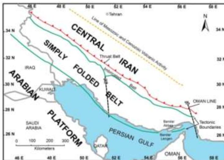
Figure 4: Tectonic settings of the Zagros fold and thrust belt showing the major tectonic belts [modified after 16]
