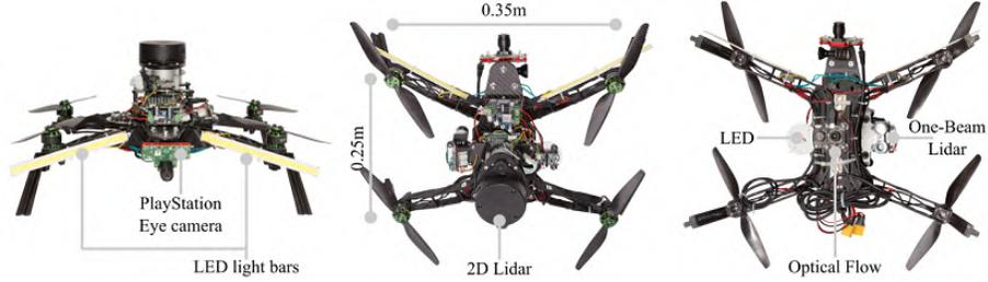
Fig. 4: The developed ROSflight based quad-copter equipped with 2D and one beam lidars, optical flow, PlayStation camera and LED bars.
