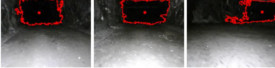
Fig. 5: Sample images of the on-board forward looking camera, while the boundary of the darkest contour is shown by red color.
