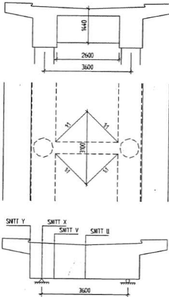
Figure D6.1. Cross beam with Sections U, V, X and Y., Leander-Fredriksson (2003), p 12:2.
