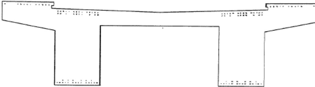
Figure D.4.1. Section M with reinforcement consisting of 110 bars  $\phi$  19 mm, page 10:5 in Leander-Fredriksson (2003),
