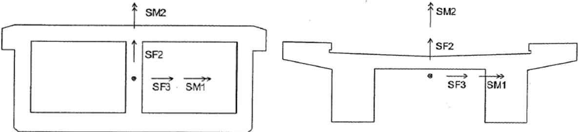
Figure D2.2 Sign conventions used for section forces for the arch (left) and the top slab and beams (right) used by Leander-Fredriksson (2003), p 8.2
