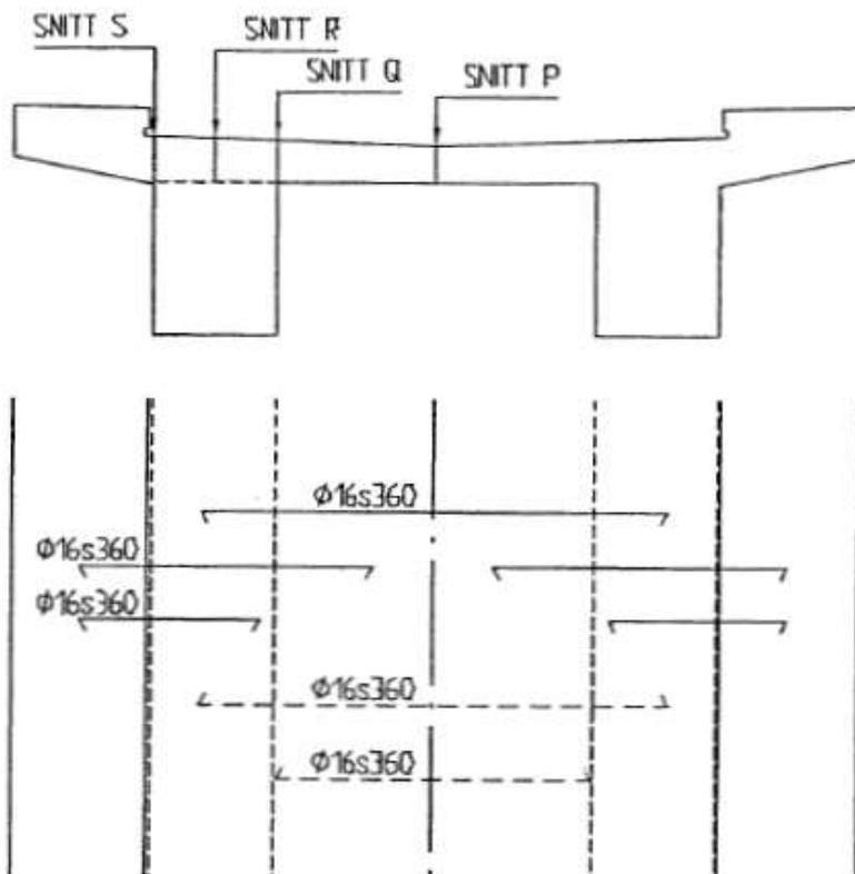
Figure D5.1. Sections of top slab controlled by Leander-Fredriksson (2003), page 11:8.
