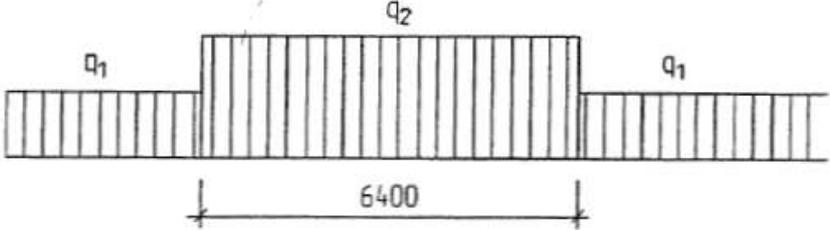
Figure D2.1. Load BV2000 as used by Leander-Fredriksson (2003), p 5:4, with  $q_1 = 116$  kN/m and  $q_2 = 217$  kN/m
