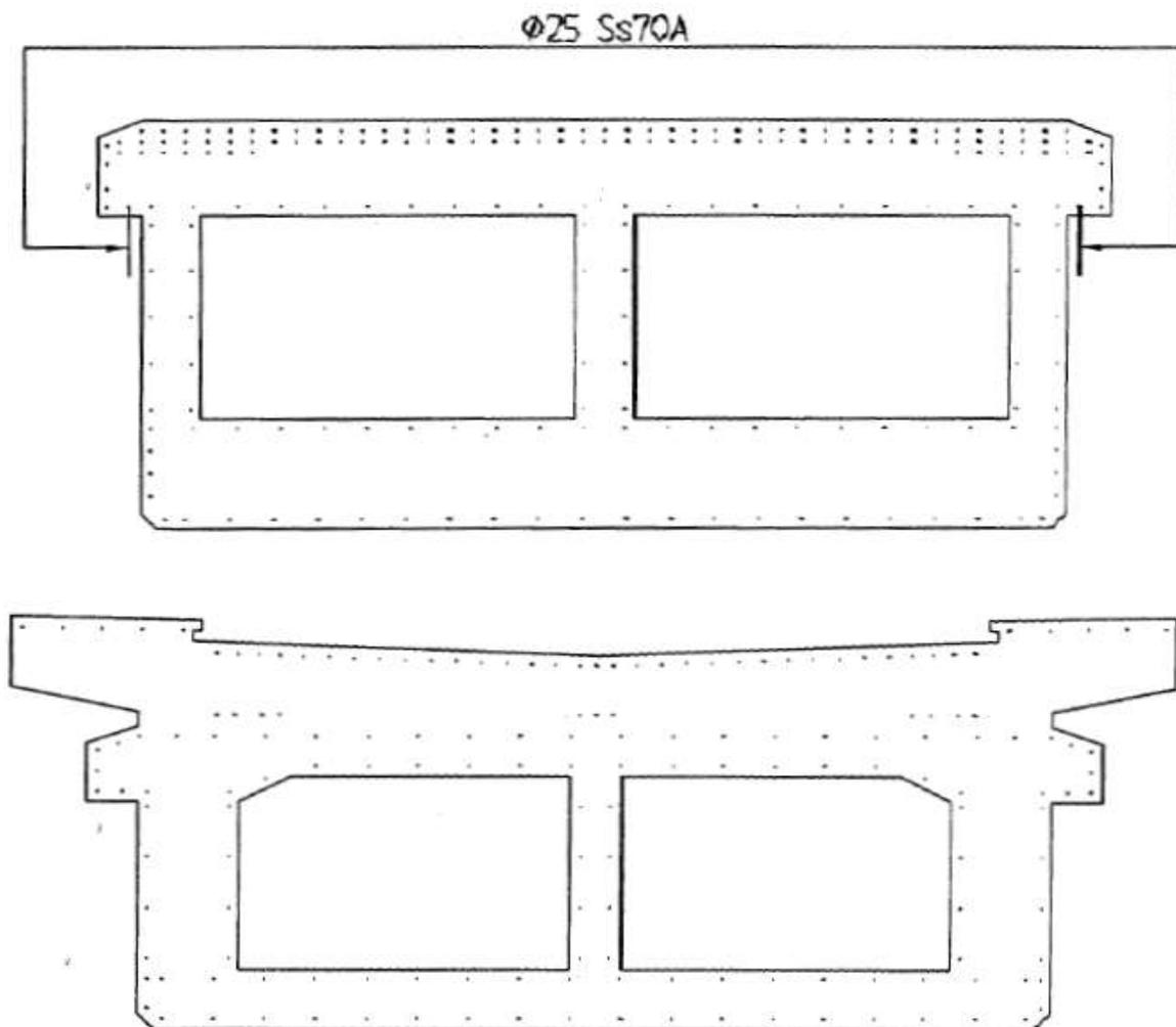
Figure D3.1 Midspan sections controlled by Leander-Fredriksson (2003). Top: Elevation, p 8:1; Middle: Section A, 112  $\phi 25$ , Ss70A ( $f_{yk} = 720$  MPa), 28  $\phi 25$  and 74  $\phi 16$  Ks 40 ( $f_{yk} = 390$  MPa) p.9:3; and Bottom: Section F, 68  $\phi 19$  and 98  $\phi 16$ , Ks 40, p 9:6.
