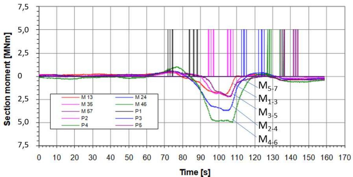
Figure E1.5. Bending moments based on the curvatures of the top beams as measured by seven LVDTs at position 1 at the top of the arch. Moment  $M_{1-3}$  indicates the moment based on the measurements in points 1, 2 and 3 and  $M_{2-4}$  is based on the points 2, 3 and 4 etc.
