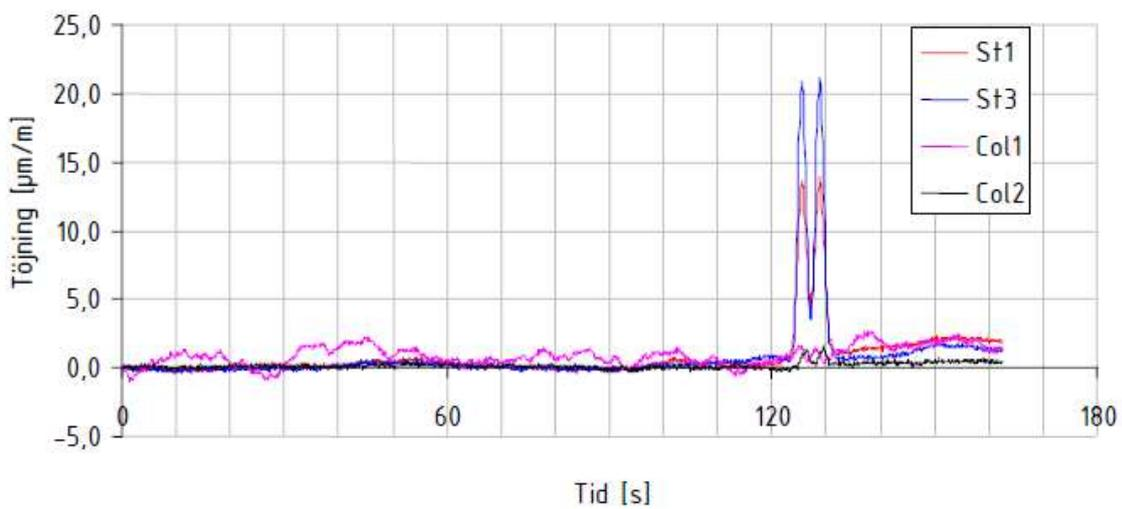
Figure E1.2. Strains in a cross-beam during passing of three train STA1-01E (top), STA2-01E (middle) and STA 3-01E (bottom). Steel strain gauges St1 and St3 and concrete strain gauges Col1 and Col 2, see Figure E1.1
