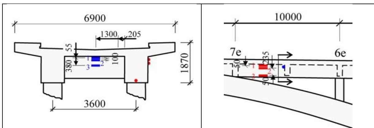
Figure E2.2. Measurements of strains. Blue gauges 1, 2 and 3 measure concrete strains in the transverse direction (CT). Red gauges 1 and 2 measure concrete strains in the longitudinal direction (CL) while red gauge 3 measures steel strains (SL) the bottom of one of the longitudinal top beams.
