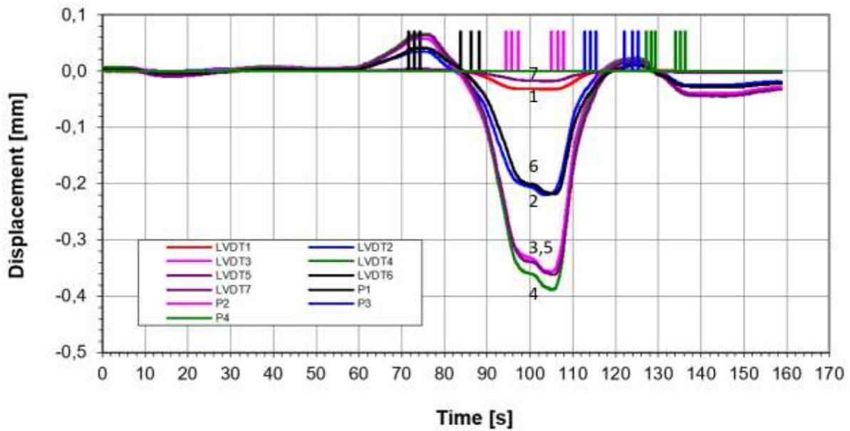
Figure E1.4. Displacements measured by seven LVDTs marked 1 – 7 in Position 1 in the centre of the arch while a train with an axle load of 210 kN is passing at a slow speed of ca 1m/sec (= 3,6 km/h). Position indicators P1-P2 show when the locomotive passes.
