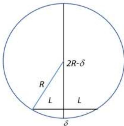
According to the chord theorem we get for a small deflection  $\delta$ , a radius of curvature  $R$  and a distance  $L$  between measurement points that
