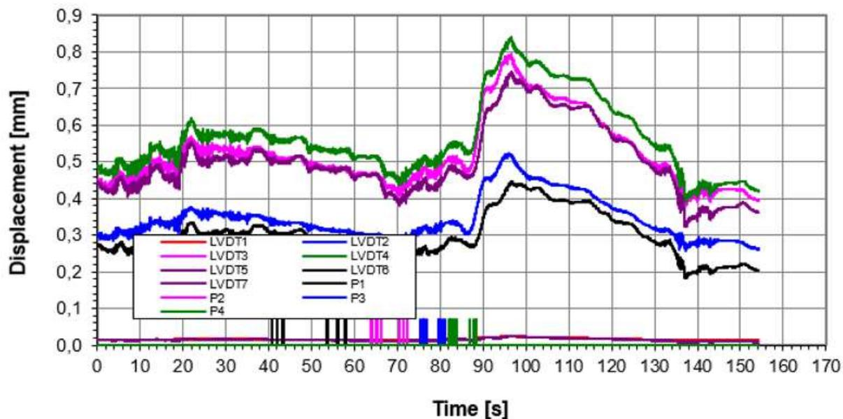
Figure E1.7. Displacements measured by seven LVDTs marked 1 – 7 in Position 3 in the centre of the arch while a train with an axle load of 210 kN is passing at a slow speed of ca 1m/sec (= 3,6 km/h). Position indicators P1-P2 show when the locomotive passes.
