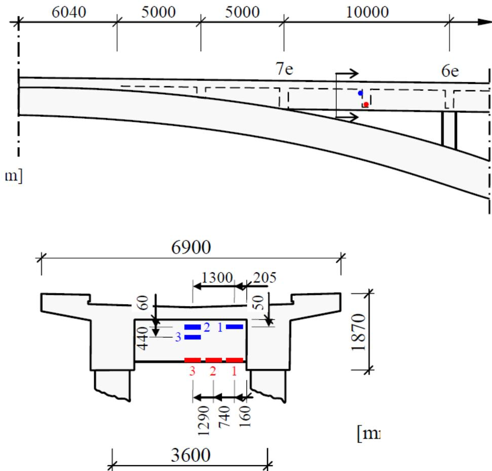
Figure E1.1 Strain gauges in a cross-beam ca 20 m from the top of the arch. Concrete strain gauges (top, blue) and steel reinforcement strain gauges (bottom, red). The gauges measure the strains in the longitudinal direction of the cross beam, i.e. in the transverse direction of the bridge...
