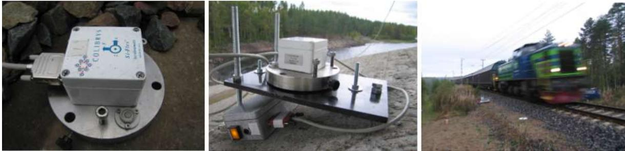
Figure E2.3. The accelerometers were firmly attached to the bridge and then aligned with a horizontal plane with three screws. The photos also show a train used for measurements
