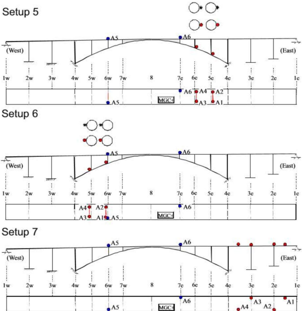
Figure E2.4. Test setups 5-7 used for acceleration measurements
