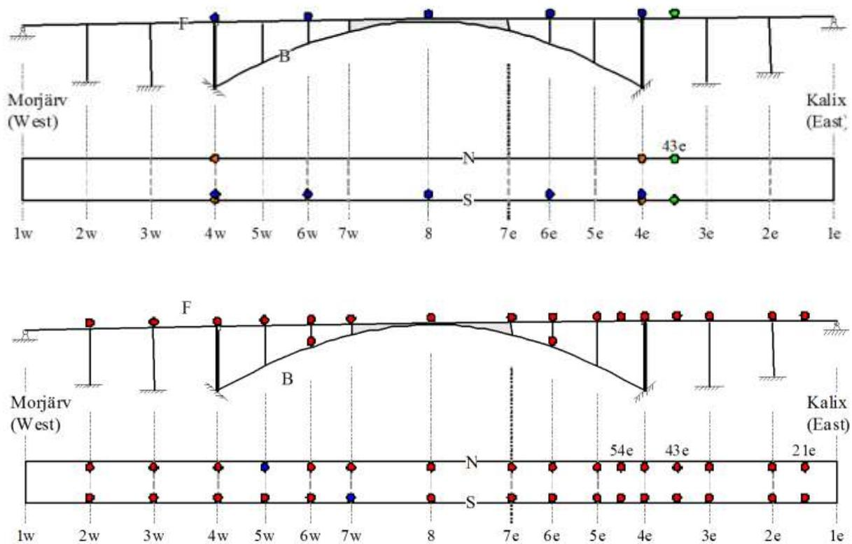
Figure E2.1. Measurements of deformations (top) and accelerations (bottom). In the top figure blue dots indicate optical measurements, green dots indicate vertical LVDTs (between 3e and 4e) and orange dots indicate horizontal LVDTs (4w & 4e). In the bottom the locations of the accelerometers are indicated
