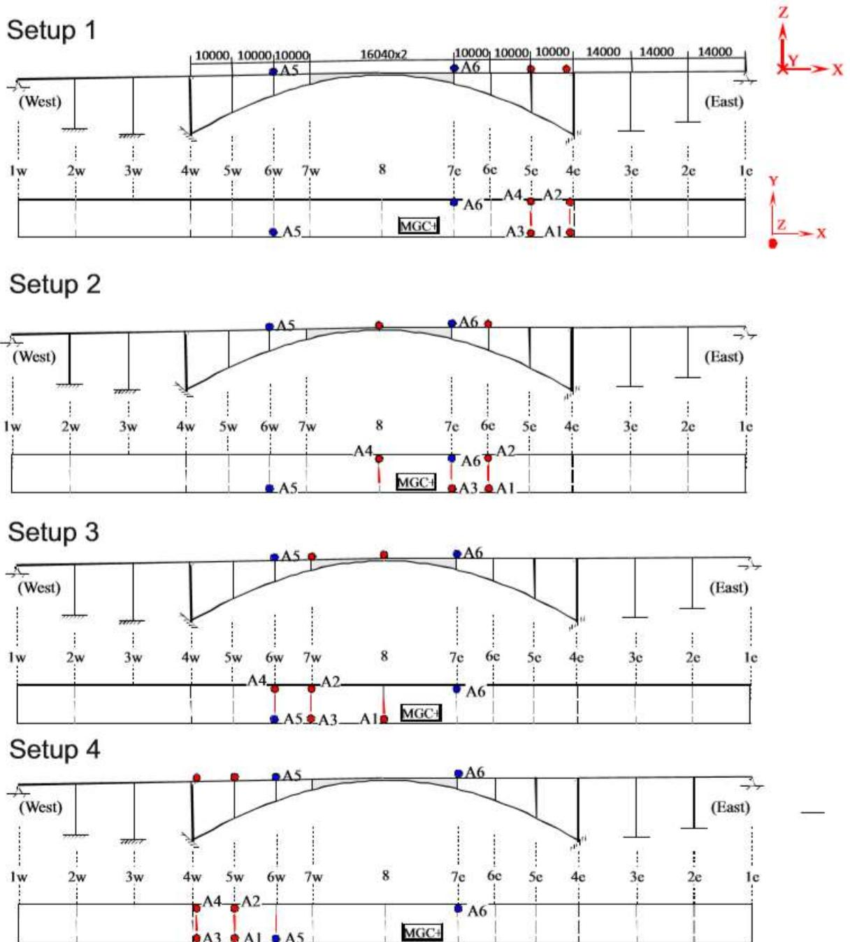
Figure E2.4. Test setups 1-4 used for acceleration measurements
