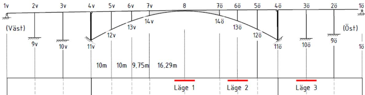
Figure E1.3. Three positions (Läge 1-3) for measurements of deflections to be used to calculate curvatures of the top beams.
