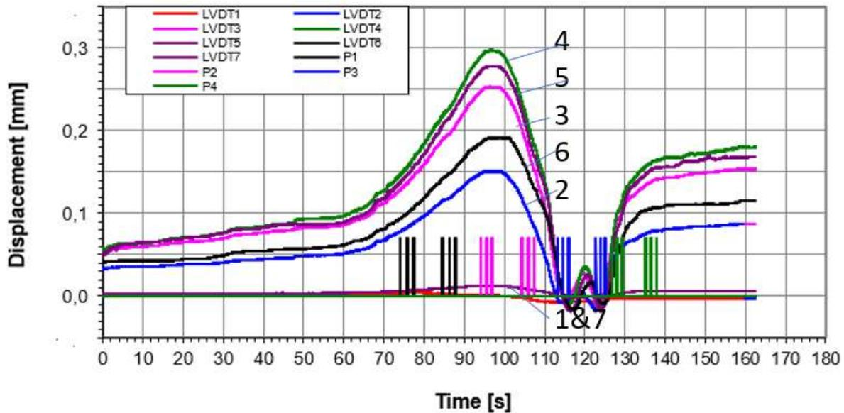
Figure E1.6. Displacements measured by seven LVDTs marked 1 – 7 in Position 2 in the centre of the arch while a train with an axle load of 210 kN is passing at a slow speed of ca 1m/sec (= 3,6 km/h). Position indicators P1-P2 show when the locomotive passes.
