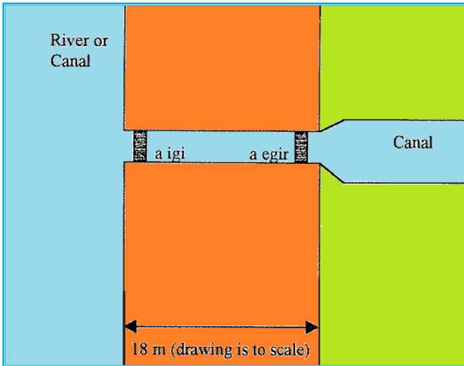
**Figure 14: Plan of regulator described in Sumerian tablet [11].**
