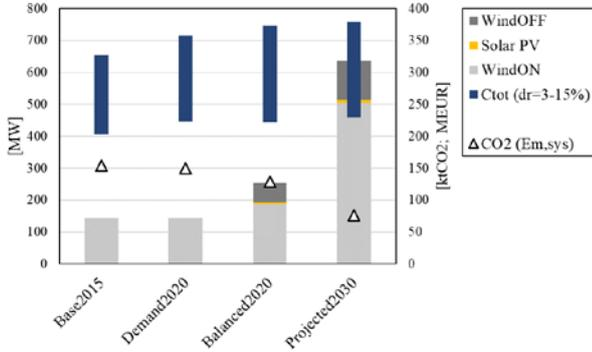
Fig. 1. Selected scenarios for the Piteå municipal energy system, simulated in EnergyPLAN. Main parameters:  $p_{el} = 40$  EUR/MWh,  $dr = 3, 9$  and  $15\%$ ; technology costs for 2015, 2020 and 2030;  $EF_{grid} = 0.156$  tCO<sub>2eq</sub>/MWh
