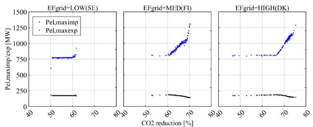
Fig. 4. Peak electricity import/export with different grid emission factors  $EF_{grid}$
