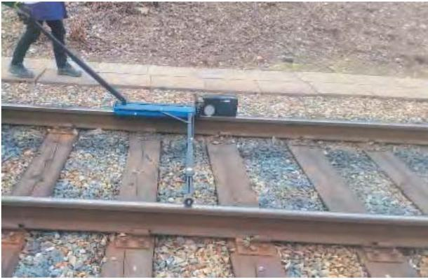
**Figure 2.** Hand push tribometer used for the friction measurements. (Photo credit: Zakarias Zouhir, Jernhusen)
