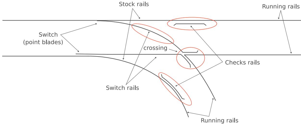
**Figure 4.** Schematic diagram showing the possible location where squeal sound can be generated.
