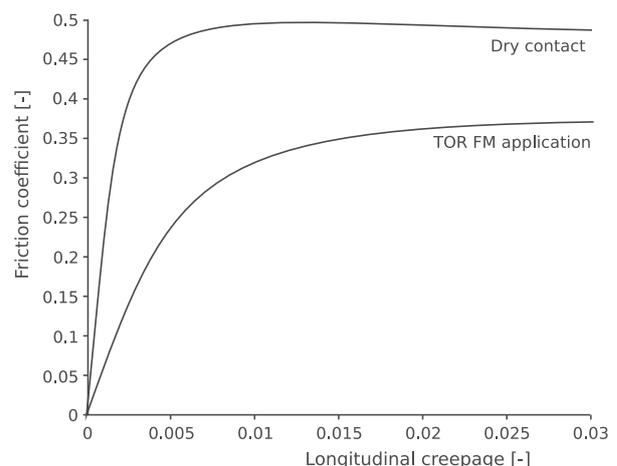
**Figure 1.** Relationship between friction coefficients and longitudinal creepage for the dry and applied-FM conditions. [7]
