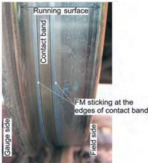
Figure 10. Image showing FM sticking on the border of the contact band.
