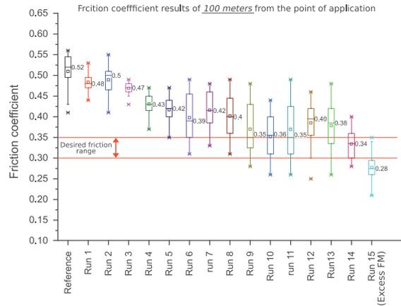
Figure 12. Friction coefficient results (box plot) of 100 meters from the point of application.
