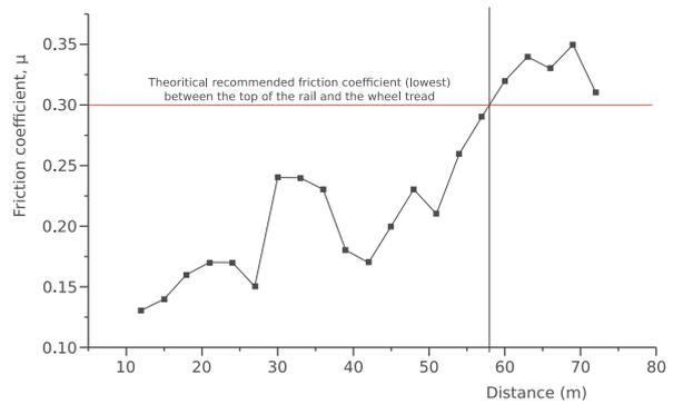
Figure 8. Friction coefficient measured using salient hand push tribometer after applying friction modifier at a location and distributed by the train
