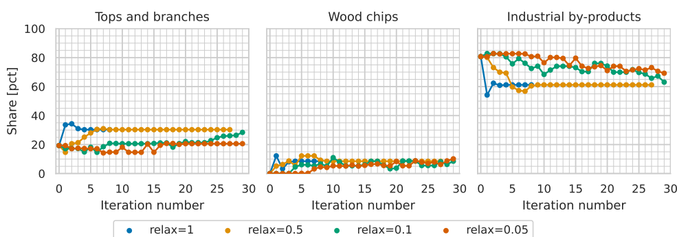
Figure 13. Biorefinery feedstock composition during the iterative process. Output from BeWhere Sweden. (Top) Config. A = using all sawmill by-products. (Bottom) Config. B = excluding the wood chips.
