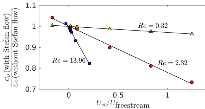
Figure 2: Normalized drag coefficient vs normalized Stefan flow velocity at different Reynolds numbers.
