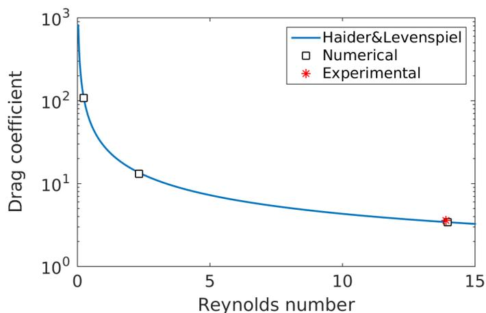
Figure 1: Drag coefficient as a function of Re no. Line: Correlation of (Haider and Levenspiel, 1989), symbols: numerical simulations and experiments.
