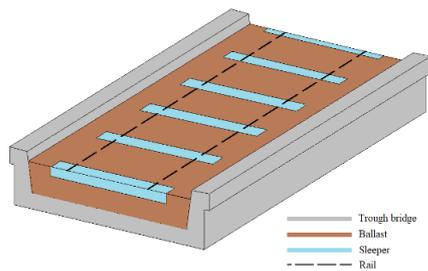
Figure 1. 3D-model of an RC trough bridge [14]
