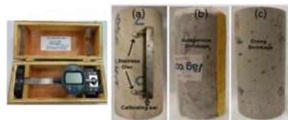
**Fig. 1.** UHPC – Autogenous and drying shrinkage test setup
