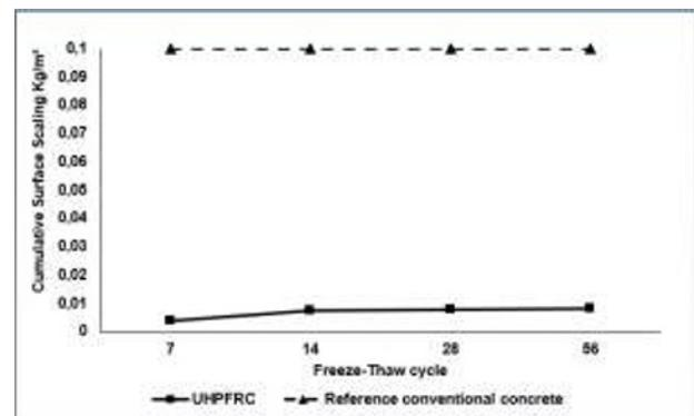
**Fig. 5.** Cumulative surface scaling of UHPC exposed to 28 F-T cycles.
