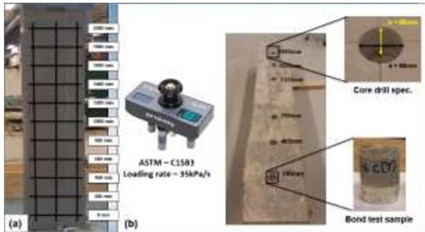
**Fig. 3.** Test setup on composite column (a) Ultrasonic pulse velocity (UPV) test nodes; (b) Pull-off test location and sample failure mode.
