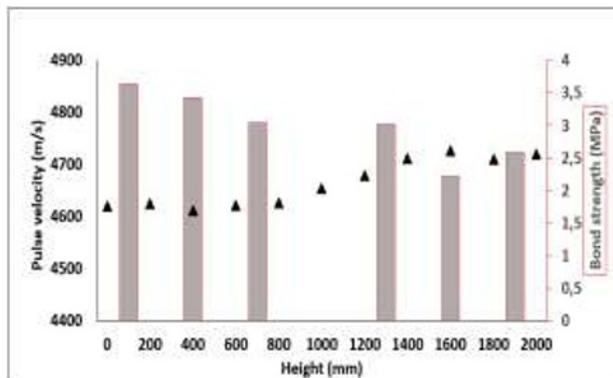
**Fig. 6.** Ultrasonic Pulse Velocity (UPV) and Pull-off test results on hybrid element (UHPC+NC) at different height.
