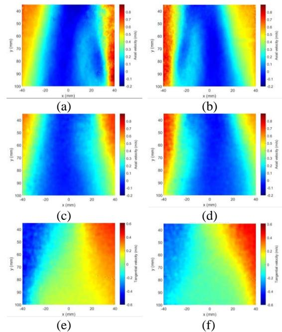
**Figure 1:** Phase averaged velocity contours in the conical section of the draft tube during PL operation. The figure on the left and right columns are separated by half of an RVR period: (a) and (b) axial velocity contours in 2D-2C PIV, (c) and (d) axial velocity contours in 2D-3C PIV, and (e) and (f) 180° apart tangential velocity contours in 2D-3C PIV.
