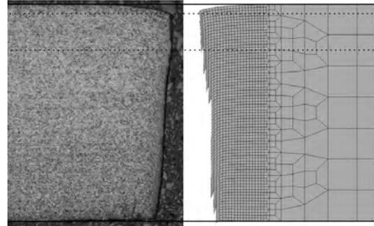
**Figure 1:** Comparison of experimental vs. numerical cut edge morphology of complex phase AHSS steel with 9% clearance.
