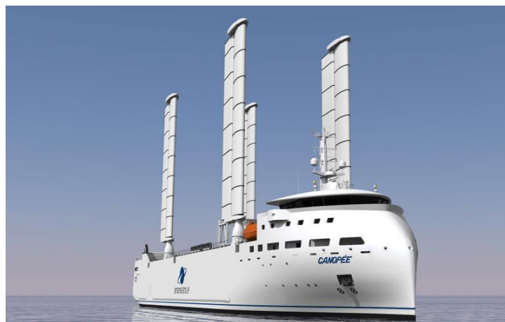
Figure 6: Example of ship equipped with hard sails (source: International Windship Association)
