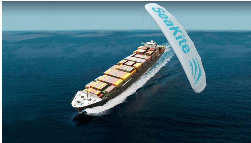
Figure 7: Use of kites to move ships
