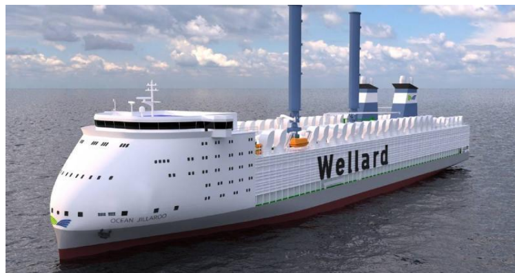
Figure 5: Flettner rotors fitted on a ship's weather deck (source: International Windship Association)
