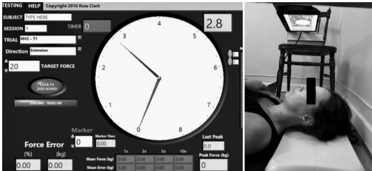
Figure 1: To the left: Visual feedback of current force of 0 kilograms and target force of 2.8 kilograms. To the right: Positioning on the WBB including the same screen above.
