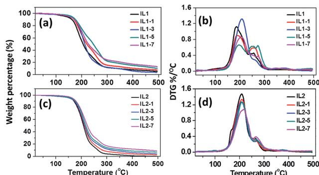
Fig. 1 (a) TGA, (b) DTG curves of lignin/[CH][AA] ILs under N<sub>2</sub> atmosphere. IL1-1, IL1-3, IL1-5 and IL1-7: 1, 3, 5, 7 wt% lignin/[choline]-[glycine]; IL2-1, IL2-3, IL2-5 and IL2-7: 1, 3, 5 and 7 wt% lignin/[choline]-[proline].
