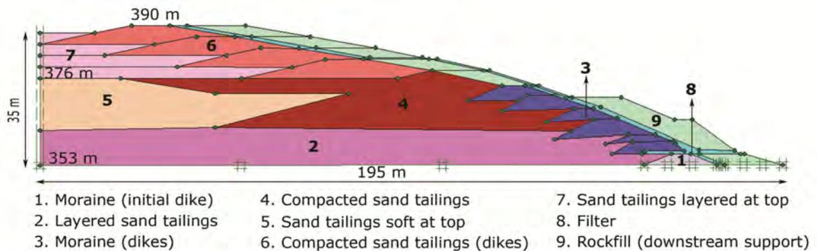
**Figure 3:** Cross section of corner E-F/G-H.
