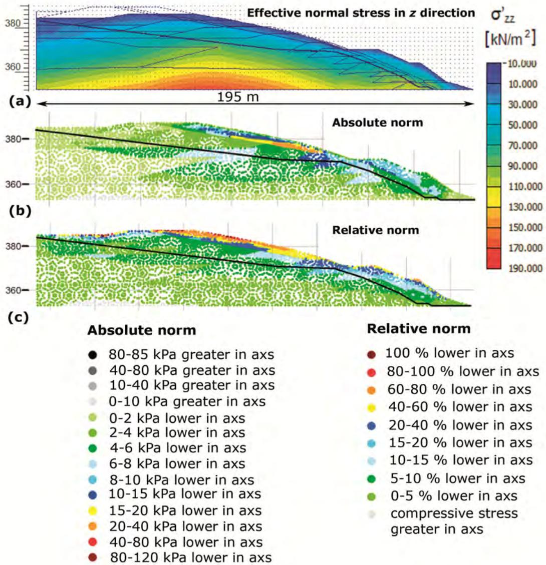
**Figure 9:** (a) Effective normal stress  $\sigma'_{zz}$  in the z direction in the axisymmetric condition (crest level +387 m). The correlation of  $\sigma'_{zz}$  for the axisymmetric and the plane strain conditions, (b) absolute norm, and (c) relative norm.
