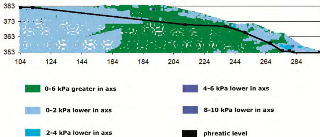
**Figure 7:** Absolute norm (difference) of the minor effective principal stress in the *x-y* plane for the axisymmetric and the plane strain conditions (crest level +384 m).
