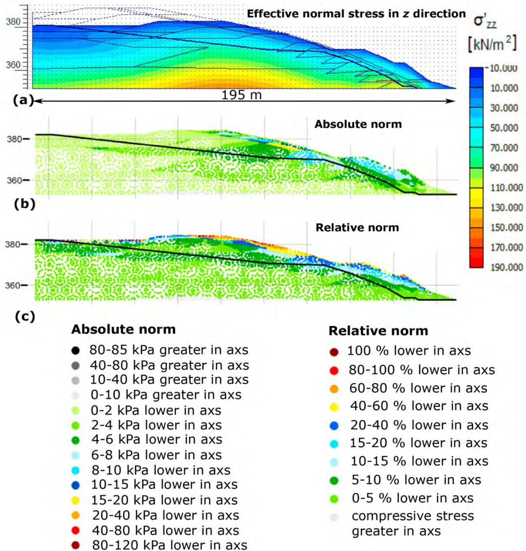
**Figure 8:** (a) Effective normal stress  $\sigma'_{zz}$  in the z direction in the axisymmetric condition (crest level +384 m). The correlation of  $\sigma'_{zz}$  for the axisymmetric and the plane strain conditions, (b) absolute norm, and (c) relative norm.
