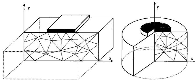
**Figure 2:** (a) Plane strain condition, and (b) Axisymmetric condition (Brinkgreve *et al.*, 2010).
