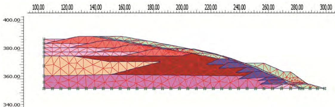
**Figure 5:** Finite element mesh of corner E-F/G-H.
