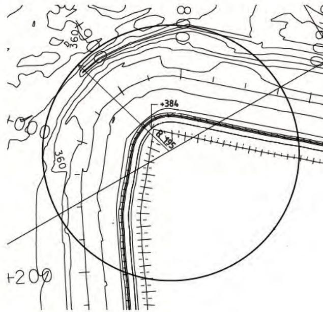
**Figure 4:** Plan of existing corner between the dam sections E-F and G-H.
