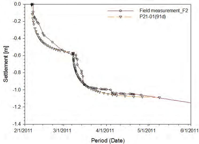
**Figure 10:** Comparison between measured values at F2 and computed settlement values from CPT point P21-01 (91d) versus time
