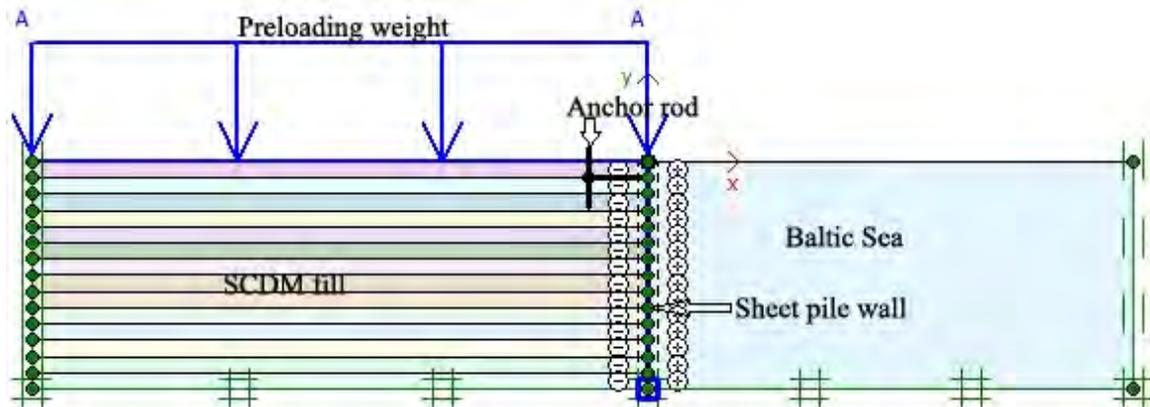
**Figure 6:** Section model showing boundary conditions for the SCDM fill (based on the CPT data at P3)
