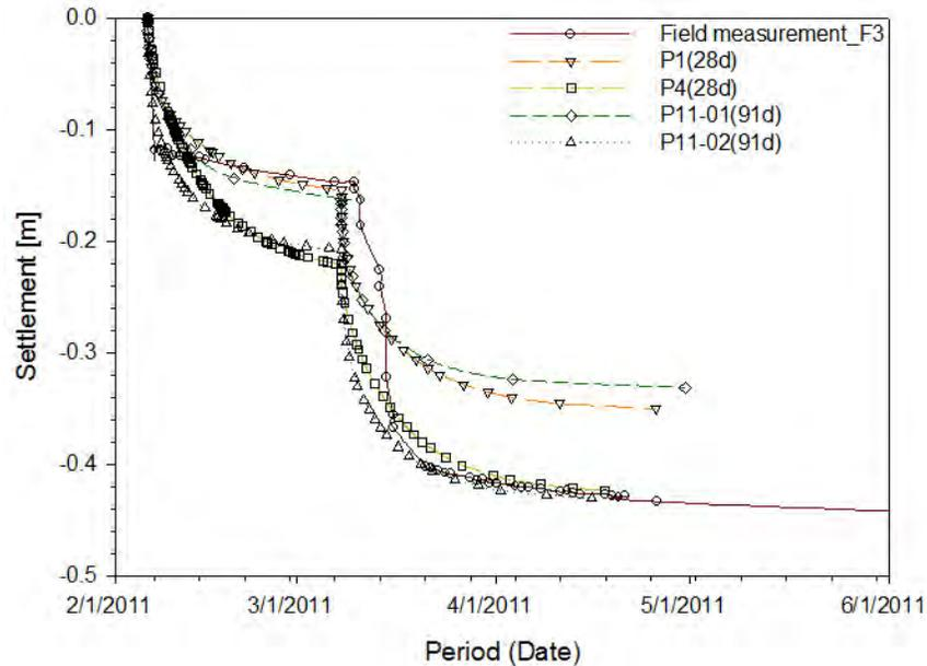
**Figure 11:** Comparison between measured values at F3 and computed settlement values from CPT point P1 (28d), P4 (28d), P11-01 (91d) and P11-02 (91d) versus time
