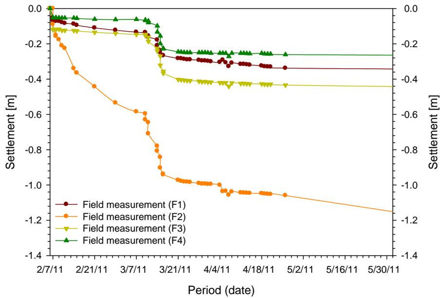
**Figure 4:** Progressive settlement measurement
