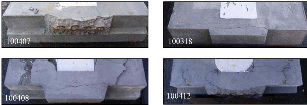
Figure 16 – Photos of shear key type 2 after failure.
