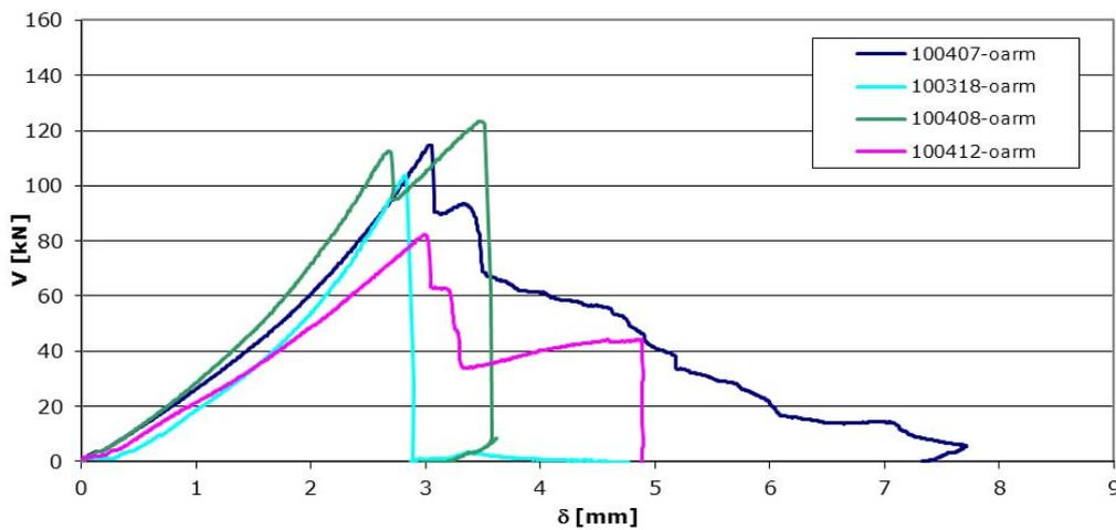
Figure 17 – Load-time curve for shear keys of type 3
