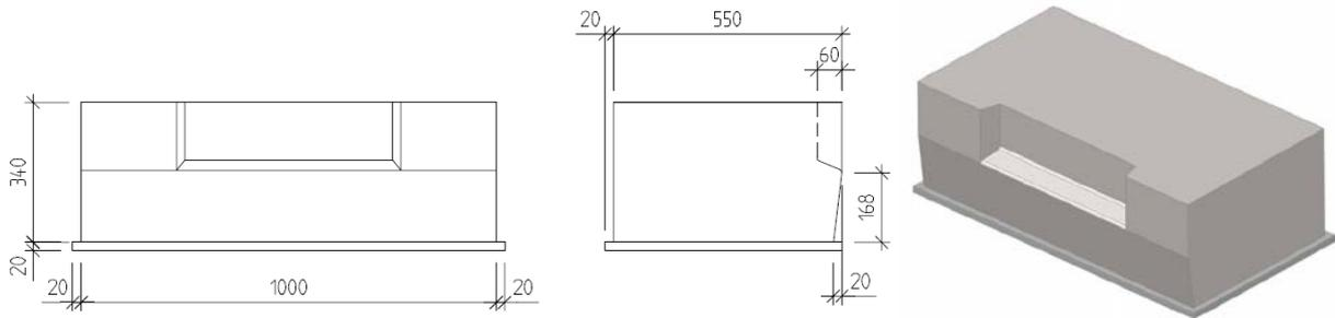
Figure 5 – Geometry drawings of support elements.
