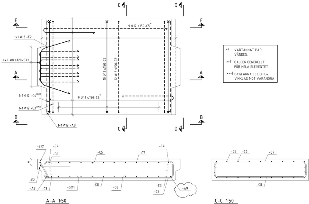
Figure 11 – Reinforcement drawing for specimens of type 2.
