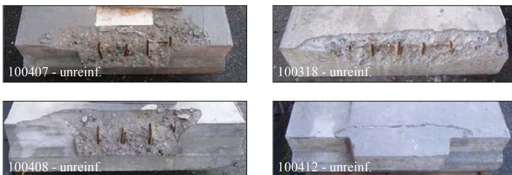
Figure 18 – Photos of shear-keys after failure.
