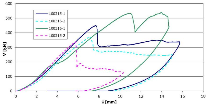
*Figure 12 – Load-deformation curve for shear key type 1, failure type 1 (solid) and 2 (dashed).*
