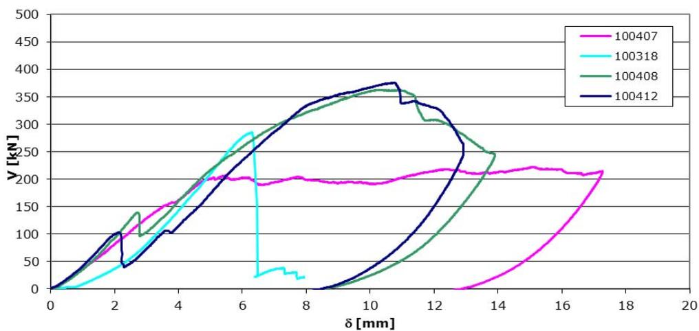
Figure 15 – Load-time curve for shear key type 2.
