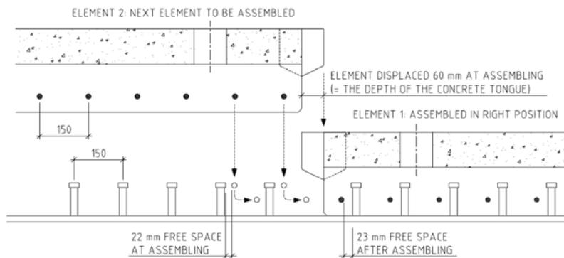
Figure 3 – Illustration of the limited tolerances. [2]
