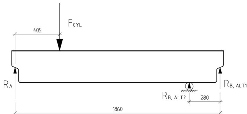
Figure 7 – Load situation with the extra support.
