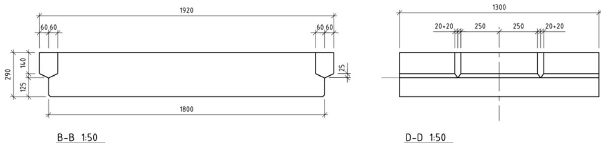
Figure 9 – General geometry of test specimens.
