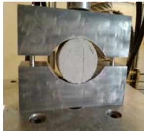
Fig. 13 Brazilian test arrangement with typical tensile fracturing [11].
