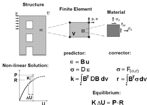
Figure 3 – Main steps of a non-linear analysis.
