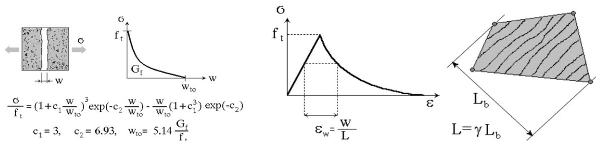
Figure 3 – Crack opening law (left). Strain softening law (middle). Crack band  $L$  (right).
