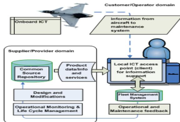
Figure 6: Illustration of an e-Maintenance concept for Information Integration
