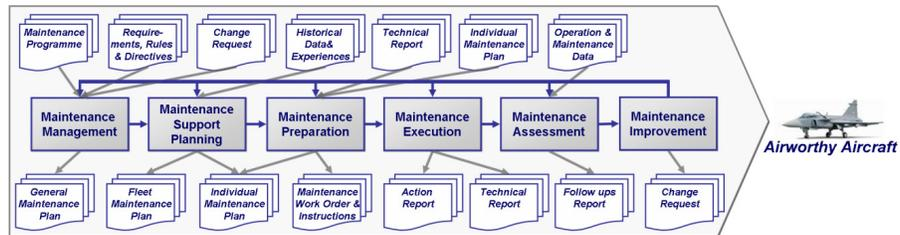
**Figure 2:** Example of Aircraft Maintenance Process
