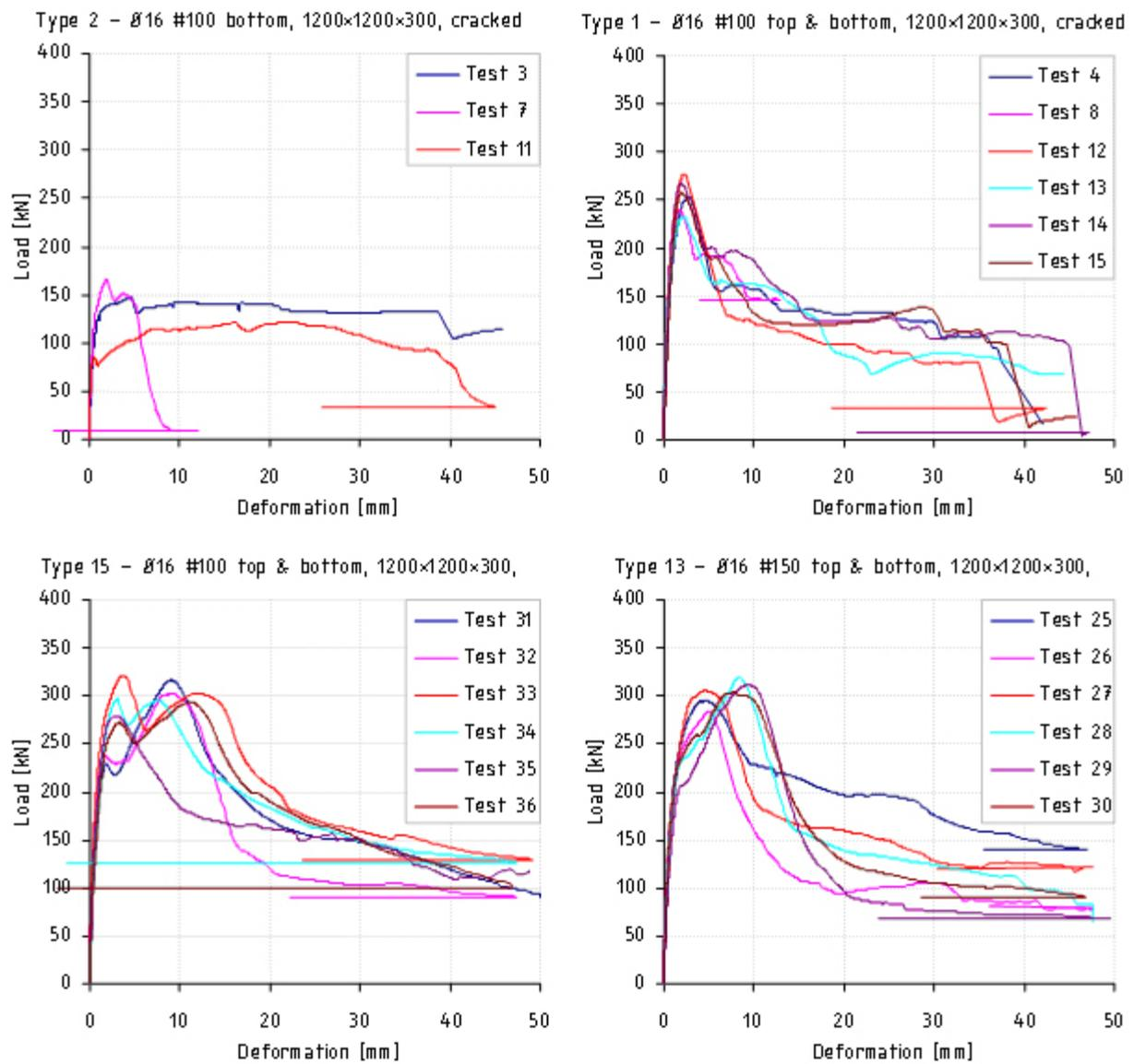
Figure 6 – Test results for slabs with cracks.
