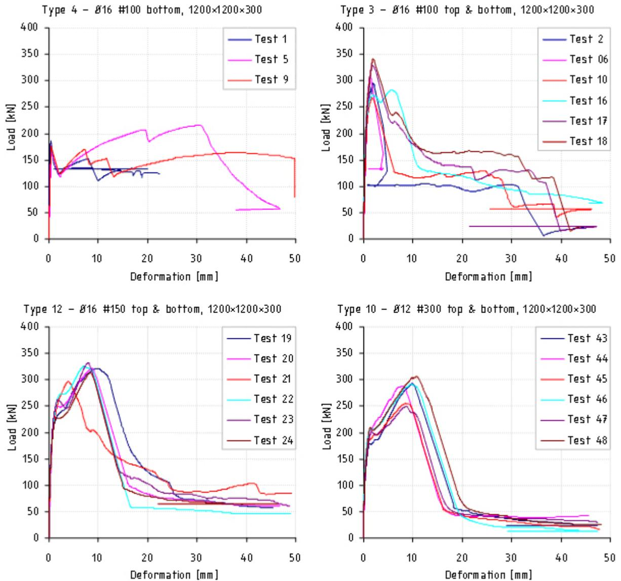
Figure 5 – Test results for slabs without cracks.
