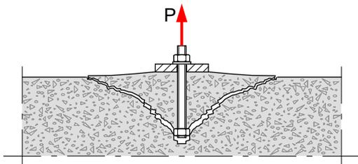
Figure 1 – Concrete cone failure.
