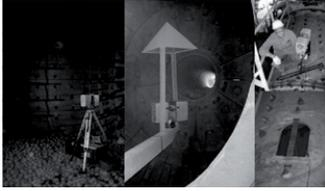
Figure 3 Terrestrial 3D laser scanners
