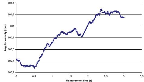
Figure 10 Angular velocity of electric motor as a function of measured time
