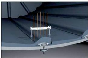
Figure 4 Mechanical wear reading device
