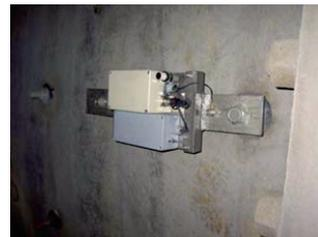
Figure 9 Device for measurement of vibrations
