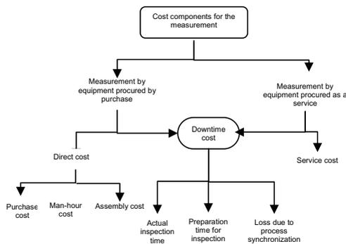
Figure 2: Overall cost structure, including the inspection cost breakdown structure, for the measuring equipment
