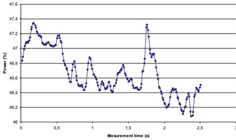
Figure 11 Percent of full power of the electric motor as a function of time
