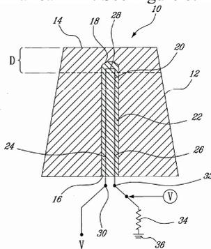
Figure 8 Measurement device inserted in liner [11]
