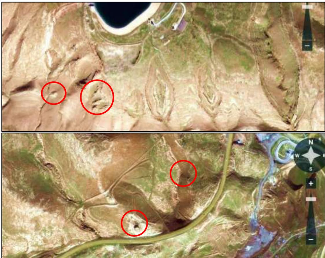
Figure 3: Flash Earth image west of Mosul Dam (Up and Down), note the developed sinkholes in the Lower Member of the Fatha Formation (encircled by red colour)
