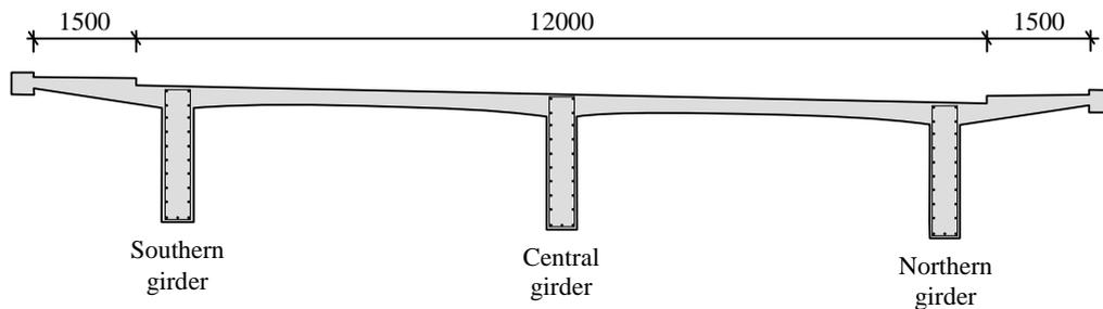
Figure 3 – Cross-section of the Kiruna Bridge.
