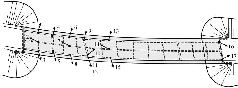
Figure 6 – Positions of bridge displacement sensors.
