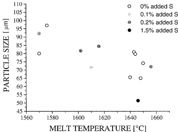
4 Estimated particle size, adjusted for water pressure, versus melt temperature
