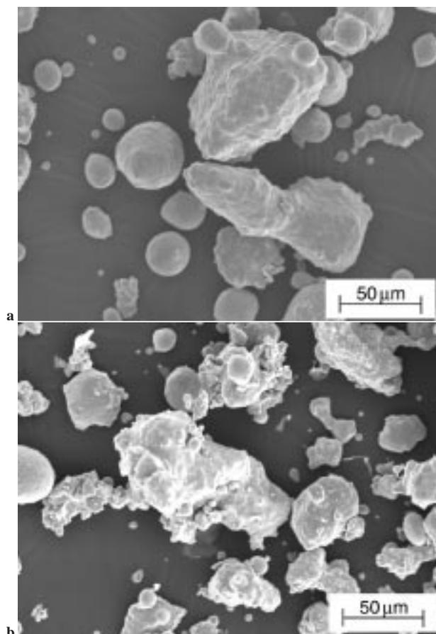
a F84, low water pressure; b F74, high water pressure
