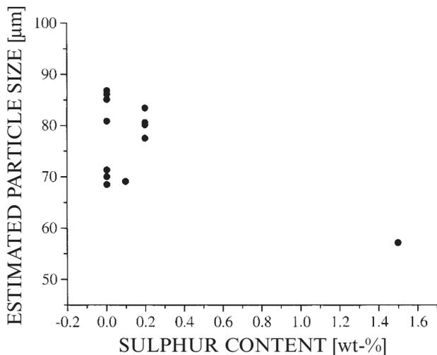
5 Estimated particle size, adjusted for water pressure and melt temperature, versus sulphur content
