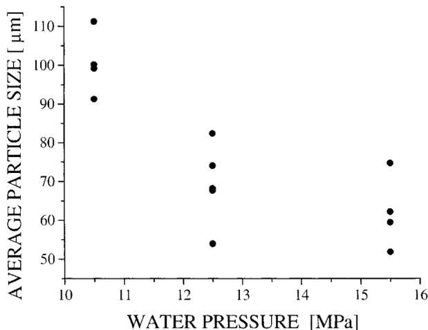
3 Resulting particle size versus water pressure
