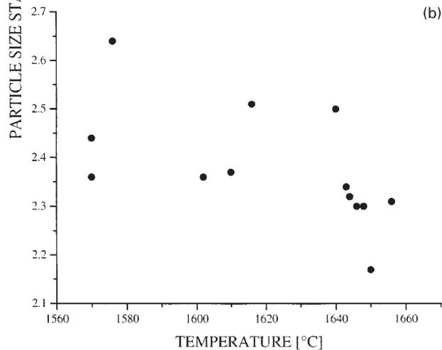
7 Particle size standard deviation versus a aluminium content and b temperature
