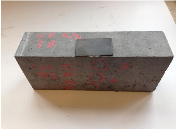
Figure 5. The cracks were locked by gluing pieces of carbon fibre to the sides of the beams.
