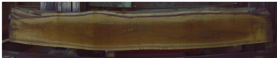
a) Board from TT sawing of Jambirre log
