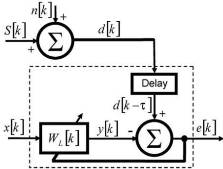
Fig. 3. Block diagram of the noise reduction filter.
