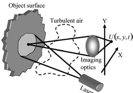
Fig. 1. Schematic of the problem. An interferometric setup measures the complex amplitude of the light from the object in an image plane as a function of time. The measurement is disturbed by a region of turbulent air between the object and imaging optics.
