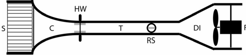
Fig 7: Sketch of the wind tunnel.
