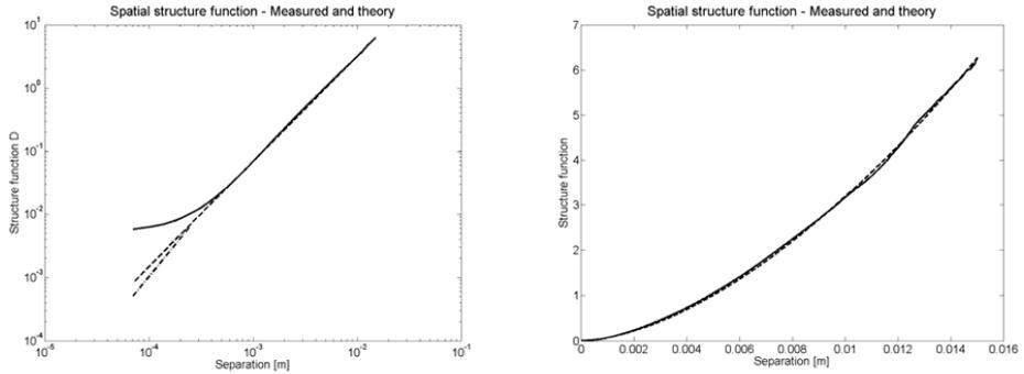
Figure 4: Spatial phase structure function with a flow velocity of 8.2 m/s and a Reynolds number of about 53000. Also shown are theoretical curves fitted from equation (2) with
