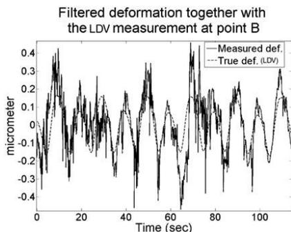
Fig. 10. Filtered deformation at B as a function of time together with the true deformation.
