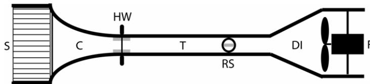
Figure 2: Sketch of the wind tunnel used to produce the turbulent air. S is the settling chamber and C the contraction cone. HW are the heated cantal wires inside the test section T. RS are the rotatable slits, DI the diffuser and F the fan.
