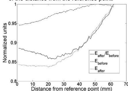
Fig. 11. Noise energy before and after filtering as a function of the distance from  $R$ . Energies are normalized so the maximum values are one. Also shown is the ratio of the noise energy after filtering to that before filtering (also normalized).
