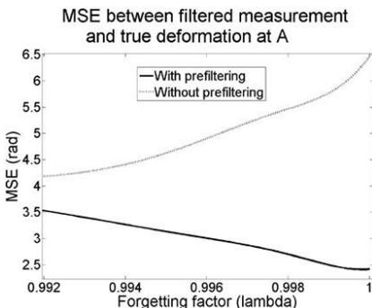
Fig. 7. MSE between the filtered measurement and true deformation as a function of the forgetting factor of the filter with and without prefiltering.
