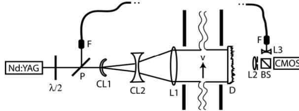
Figure 1: Sketch of the experimental setup.  $\lambda/2$  is a halfwave plate and P is a thin film polarizer. CL1 and CL2 are cylindrical lenses and L1,L2,L3 are ordinary single lenses. D is a diffuser plate and BS a beamsplitter cube. CMOS is the high-speed camera.
