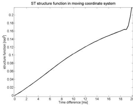
Figure 7: ST phase structure function at zero separation in a coordinate system moving along with the flow.
