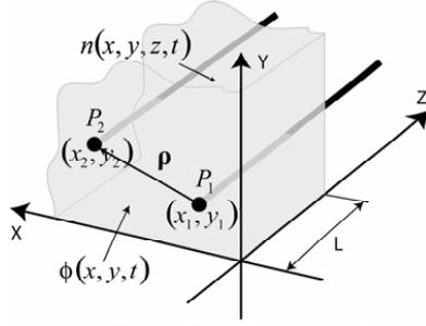
Figure 3: Light propagation geometry. The refractive index fluctuations in the turbulent region of size  $L$  are  $n(x, y, z, t)$ .  $\phi(x, y, t)$  is the phase fluctuations of the wave in the detector plane.  $\rho$  is the vector between two points  $P_1$  and  $P_2$  in the detection plane with coordinates  $(x_1, y_1)$ ,  $(x_2, y_2)$ .
