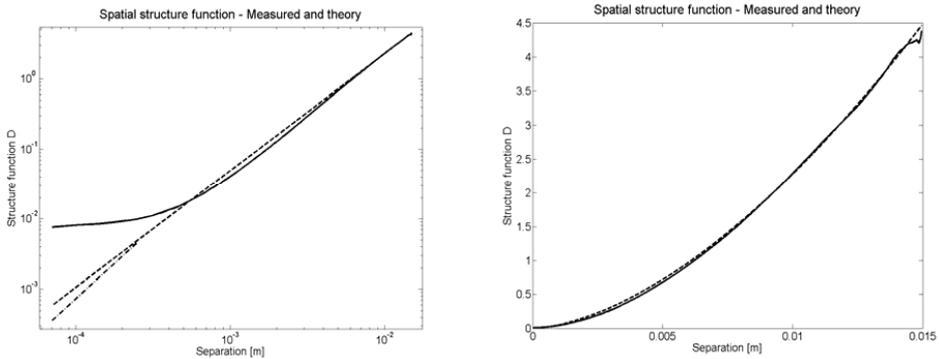
Figure 5: Spatial phase structure function with a flow velocity of 2.7 m/s and a Reynolds number of 18000. Also shown are theoretical curves fitted from equation (2) with
