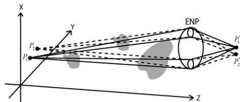
Fig. 2. Connection between the phase changes at an image point and the refractive index distribution of the turbulent air.
