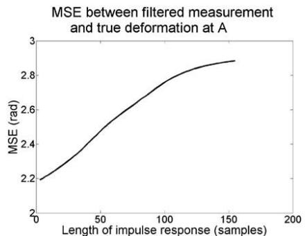
Fig. 8. MSE between the filtered measurement and true deformation as a function of the impulse response length of the filter.
