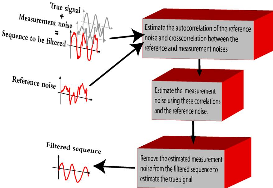
**Fig 6:** Procedure for filtering the time sequences.
