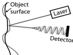
**Fig 3:** *Basic principle of holographic interferometry*
