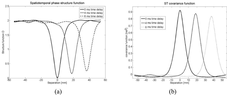
Figure 6: ST phase structure and covariance function for a flow velocity of 4.6 m/s.
