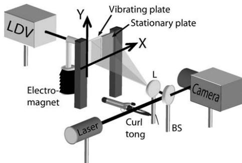
Fig. 4. Schematic of the experimental setup.
