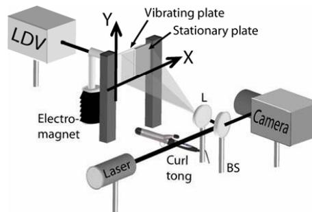
**Fig 4:** Sketch of the measurement setup
