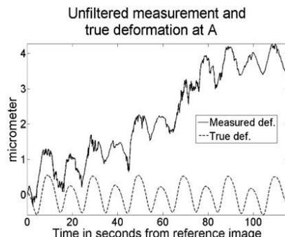
Fig. 6. Unfiltered deformation at point  $A$  as a function of time (see Fig. 5) together with the true deformation.
