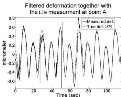
Fig. 9. Filtered deformation at A as a function of time together with the true deformation.
