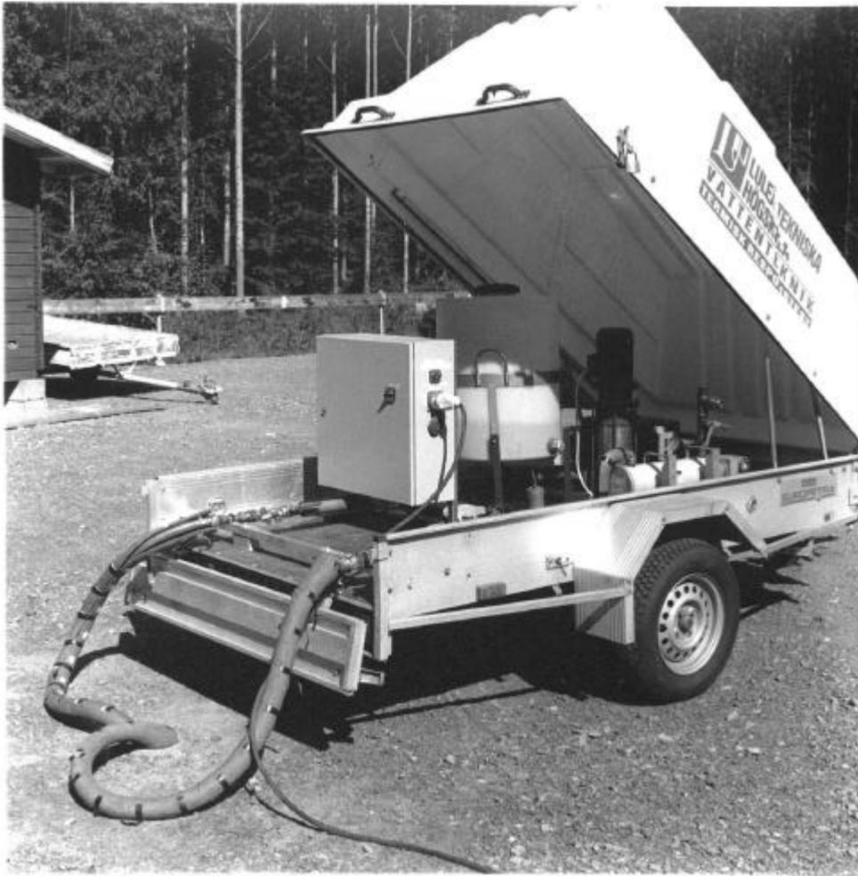
Figure 5. The thermal response test equipment - TED, 1998. Photo: Peter Olsson.
