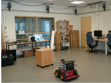
Figure 6: Experimental setup used for recording the dataset. The Lidar was mounted over a Pioneer 3AT robot facing an obstacle; the photo moreover shows some of the cameras of the MoCap system.
