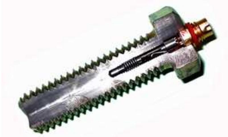
Figure 2: Hitec corporation approach to the measurement of bolt load with an insert to the bolt head.
