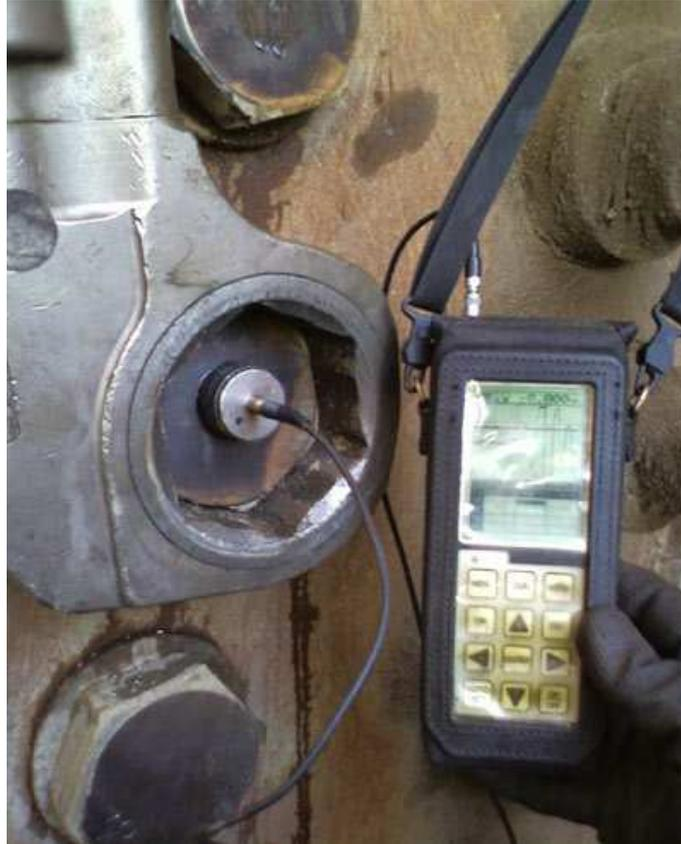
Figure 5: Ultrasonic bolt load measurement technology USM-3 by Nobar.
