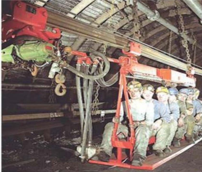
**Figure 6.** Personnel transportation using monorail (Scharf, 2007)
