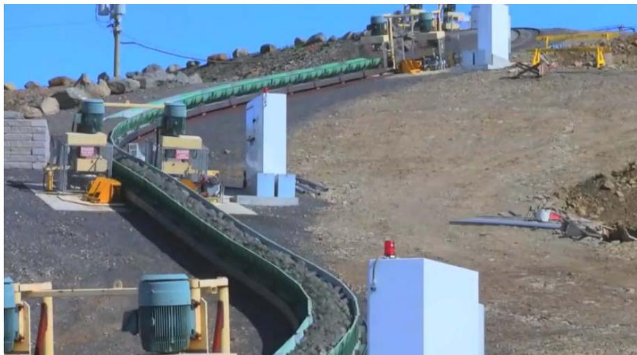
**Figure 8.** Material transportation on rail-veyor (<http://www.railveyor.com/>)
