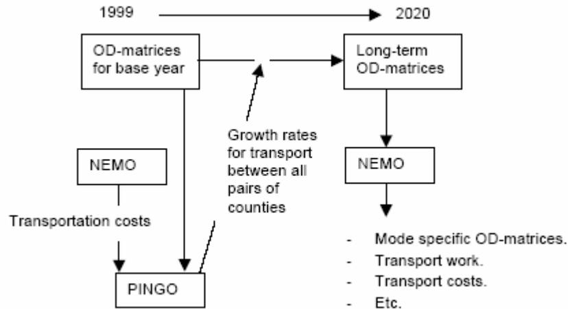
Figure 1. A schematic view of the interplay between NEMO and PINGO. (From TÖI report 578/2002).
