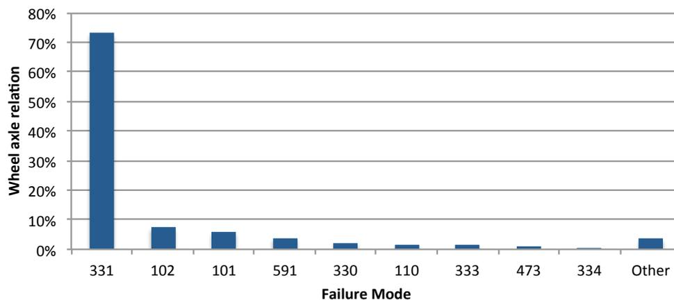
Figure 3.1: Wheel axles split into major failure modes with 26 less frequent failure modes as Other.
