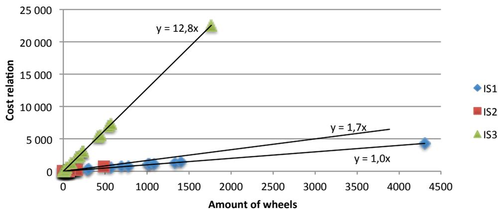
Figure 3.4: Scatter plot presenting the cost for a specific number of maintained wheel axles with the addition of a trend line.
