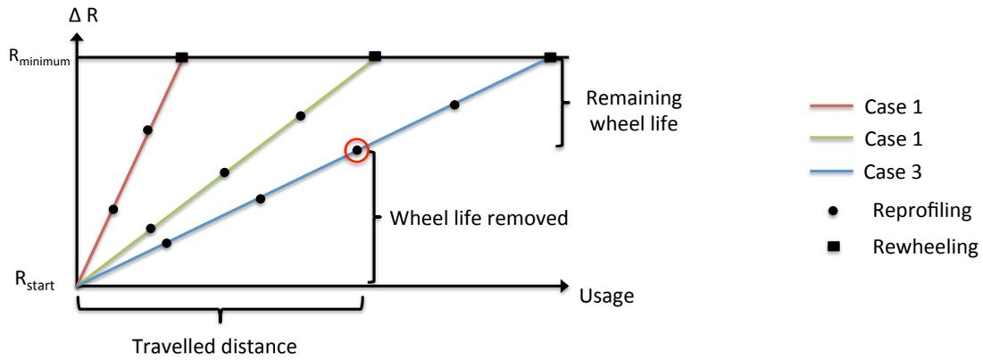
Figure 3.8: Three different life lengths of wheel axles with different amounts of ISI and one re-profiling
