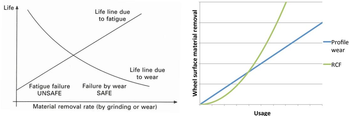
Figure 3.6a: Rail life vs material removal. [Ref. 4, pp.52]
