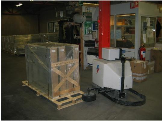
**Figure 11: Packing of glass doors**
