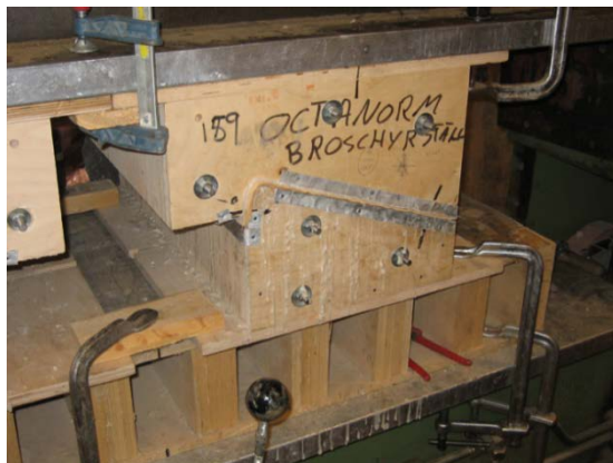
a) Figure 3. a) Mould where the shell was laminated, and b) stance for newly pressed shells.
