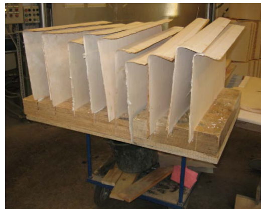
a) Figure 3. a) Mould where the shell was laminated, and b) stance for newly pressed shells.
