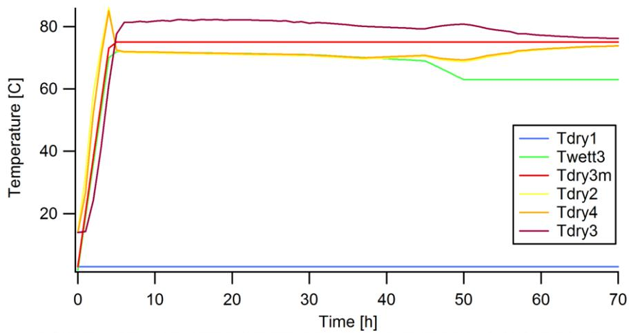
FIGURE 6 - DRY AND WET BULB TEMPERATURE IN THE DRYING CYCLE POINT 1-4
