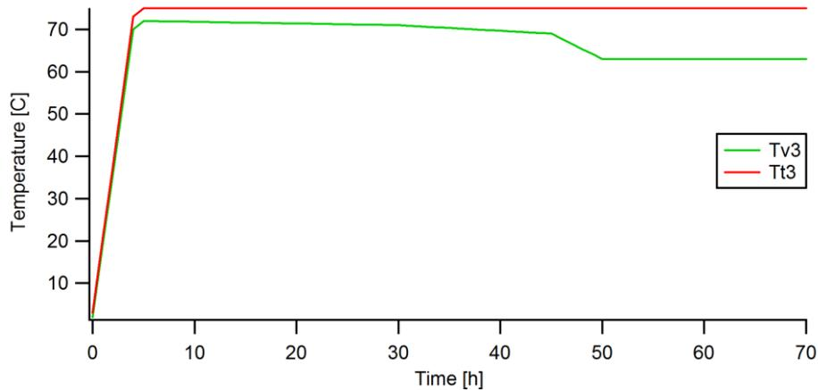
FIGURE 4 - TORKSIM PROVIDED SCHEME FOR DRY AND WET BULB TEMPERATURE OVER TIME
