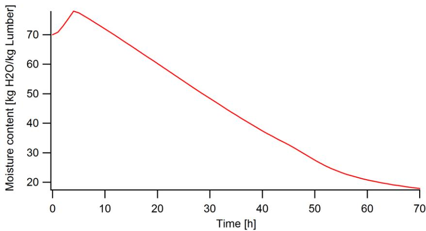
FIGURE 5 - TORKSIM PROVIDED SCHEME OF MOISTURE CONTENT OVER TIME
