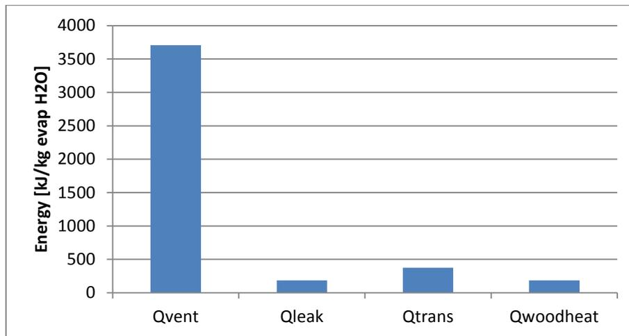
FIGURE 10 - USED ENERGY PER KG EVAPORATED WATER
