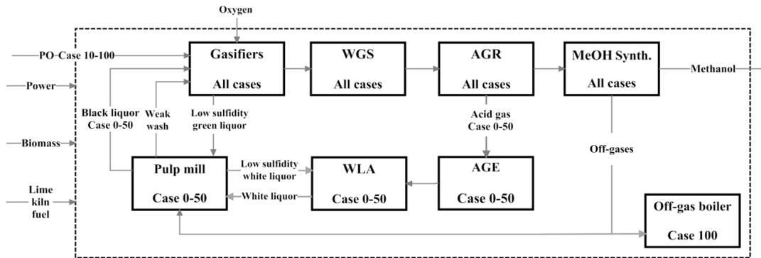
**Figure 1.** Simplified flowsheet for the different methanol production pathway.
