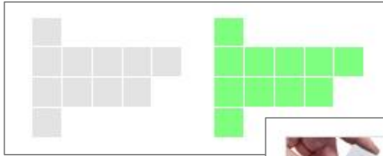
Figure 2:19 To the left is the pixels sent from the rasterizer. To the right is the pixels colored after the pixel shader.
