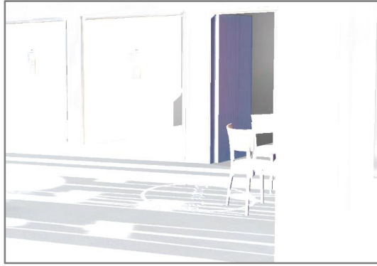
Figure 4:16 Subtraction between baked and real-time shadows to find pixels are affected. Deleting all white pixels and comparing pixels to determinate the percent.
