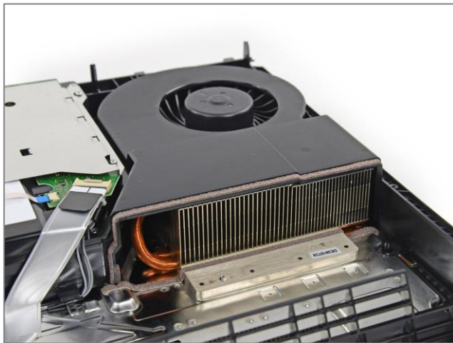
Figure 2:7 PlayStation 4 APU cooler VII
