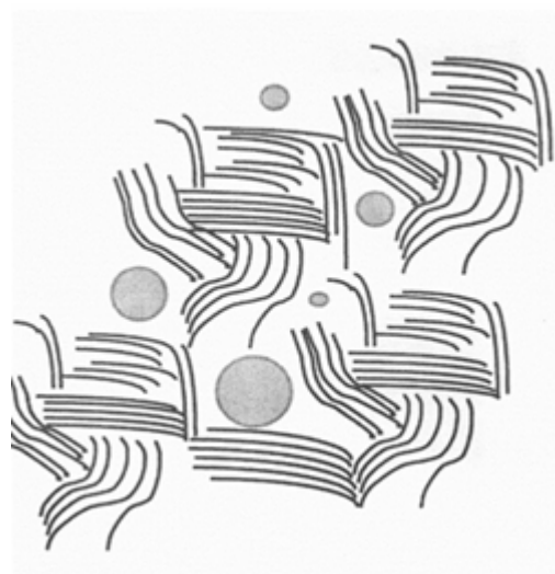
Figure 2. Microstructural voids with DW droplets between 3-7 nm thick stacks of smectite lamellae in uncompacted air-dry smectite clay (Pusch, 2015).
