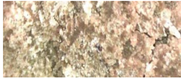
Figure 5. Holmehus clay microstructure. Optical micrograph of moist DW-saturated clay with 1570 kg/m 3 wet density (magnification 250x).
