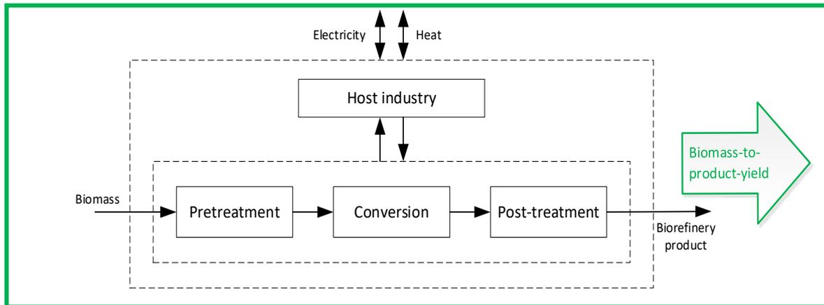
**Figure 3.** Overview of the system boundaries for techno-economic evaluation of a generic, host-integrated, thermo-chemical biorefinery.
