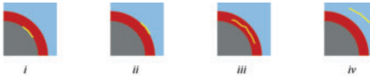
Figure 27. Possible damage initiation sites along the test specimen, at i ) fiber/coating, ii ) coating/matrix interfaces, in the iii ) coating and iv ) matrix.
