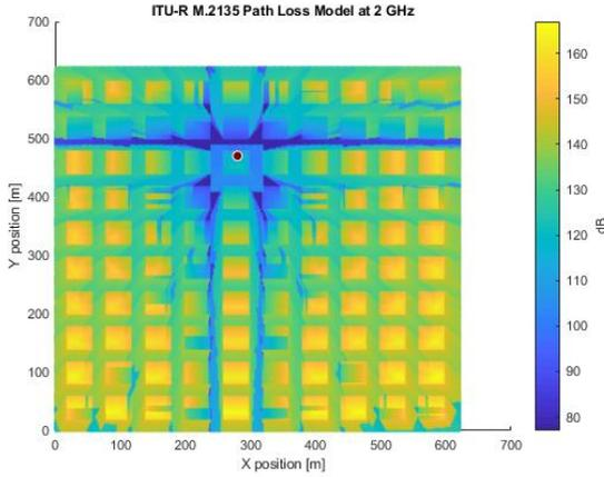
Fig. 2: Path Loss Map for a LTE macro base station
