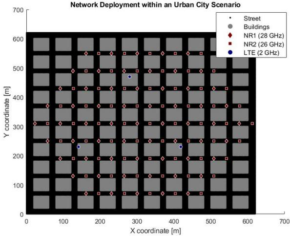
Fig. 1: UDN deployed in the Manhattan Grid
