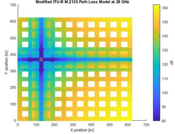
Fig. 3: Path Loss Map for a NR micro base station
