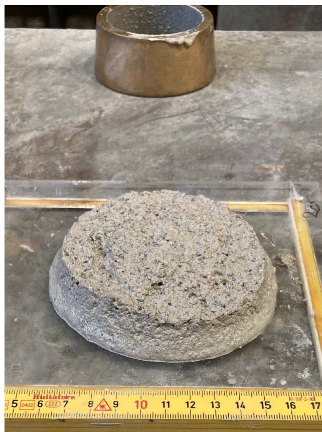
Figure 1. Mini-slump flow test. The measurement was done on the bottom diameter of the LMG material. Consistency in the figure is approximately 100 mm
